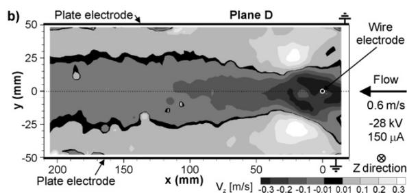
**Fig. 12** Averaged flow velocity field in the Plane A in the ESP. Negative voltage of -28 kV was applied. EHD number was  $4.7 \times 10^7$  and  $Ehd/Re^2$  was 3.2
