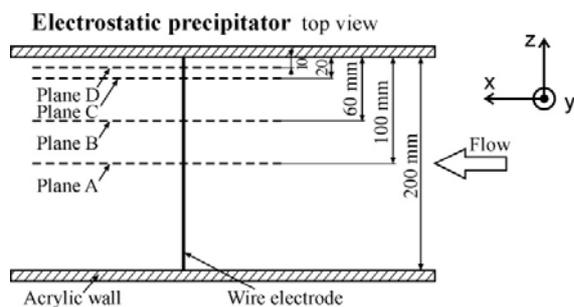
**Fig. 2** ESP top view. Measurement planes A, B, C and D marked by dashed lines
