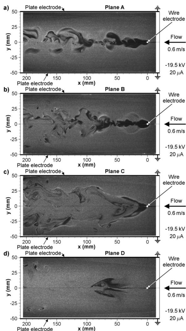
**Fig. 7** Instantaneous images of the flow in the planes A, B, C and D in the ESP when negative voltage of -19.5 kV was applied. EHD number was  $6.2 \times 10^6$  and  $Ehd/Re^2$  ratio was 0.43. Exposure time: 6 ns
