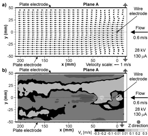
**Fig. 9** Averaged flow velocity field in the Plane A in the ESP. Positive voltage of 28 kV was applied. EHD number was  $5.5 \times 10^7$  and  $Ehd/Re^2$  was 3.75
