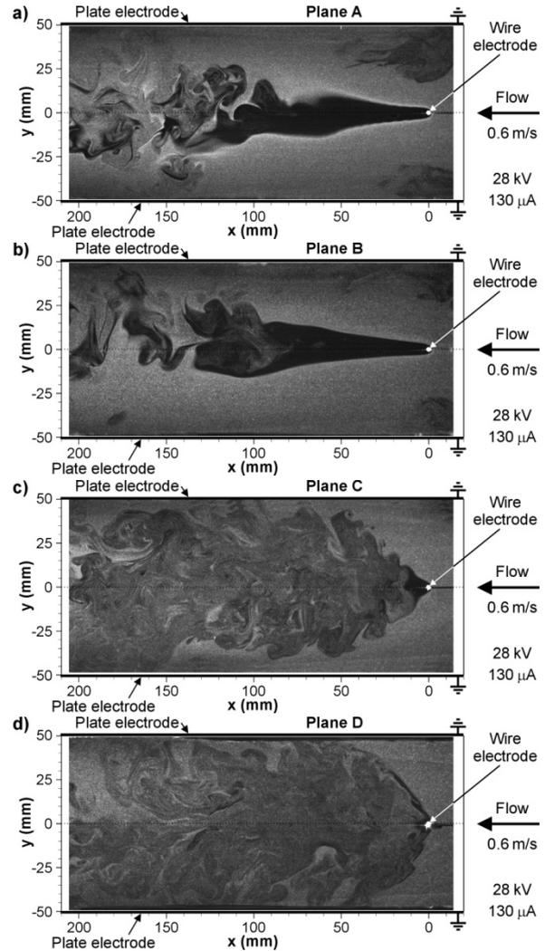
**Fig. 6** Instantaneous images of the flow in the planes A, B, C and D in the ESP when positive voltage of 28 kV was applied. EHD number was  $5.5 \times 10^7$  and  $Ehd/Re^2$  was 3.75. Exposure time: 6 ns
