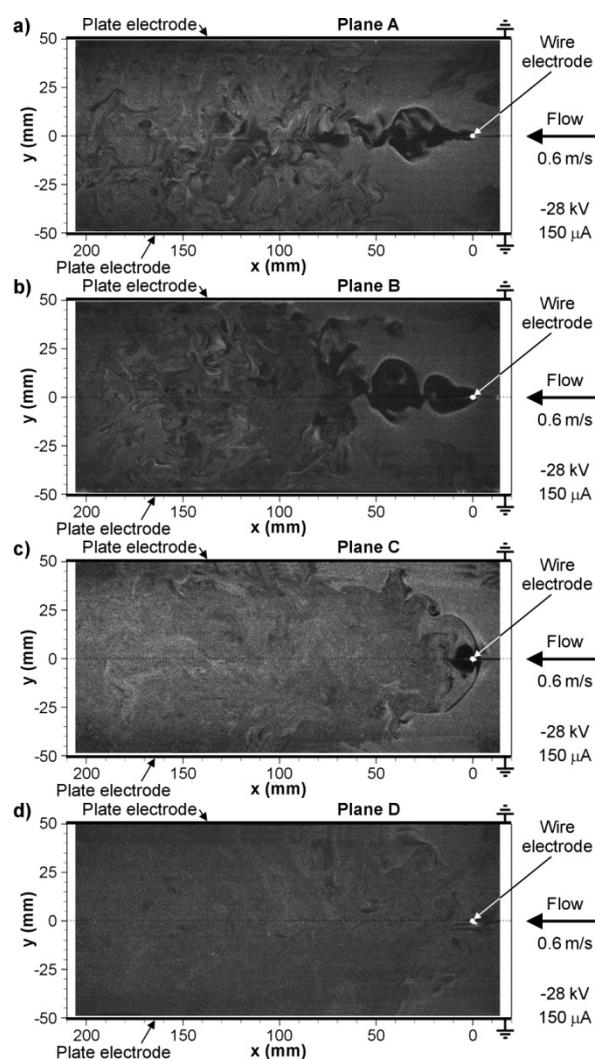
**Fig. 8** Instantaneous images of the flow in the planes A, B, C and D in the ESP when negative voltage of -28 kV was applied. EHD number was  $4.7 \times 10^7$  and  $Ehd/Re^2$  was 3.2. Exposure time: 6 ns
