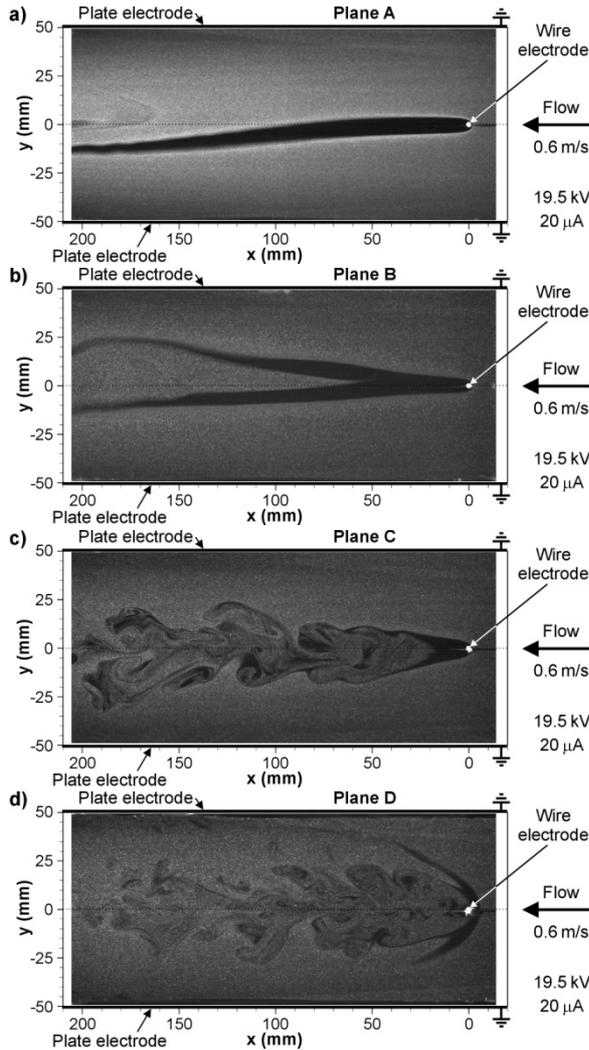
**Fig. 5** Instantaneous images of the flow in the planes A, B, C and D in the ESP when positive voltage of 19.5 kV was applied. EHD number was  $8.4 \times 10^6$  and  $Ehd/Re^2$  was 0.57. Exposure time: 6 ns
