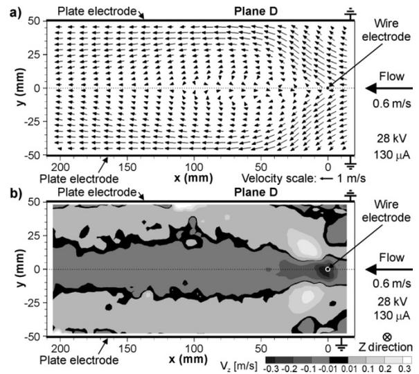
**Fig. 11** Averaged flow velocity field in the Plane D in the ESP. Positive voltage of 28 kV was applied. EHD number was  $5.5 \times 10^7$  and  $Ehd/Re^2$  was 3.75.
