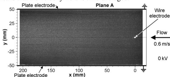
**Fig. 3** Instantaneous image of the flow in the ESP when no voltage was applied. Exposure time: 6 ns
