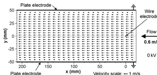
**Fig. 4** Averaged flow velocity field in the Plane A in the ESP when no voltage was applied
