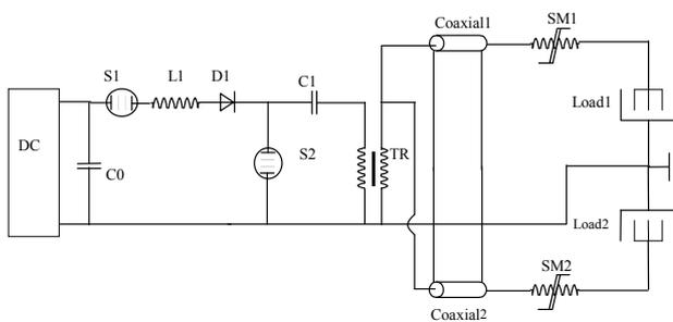
DC-power supply; C<sub>0</sub>-energy storage capacitor; S(1,2)-thyratrons L<sub>c</sub>-inductance; D1-diode stack; C1-pulsed capacitor TR-pulsed transformer; Coaxial(1,2)-coaxial cables SM(1,2)-magnetic pulsed compressors Load(1,2)-reactor loads
