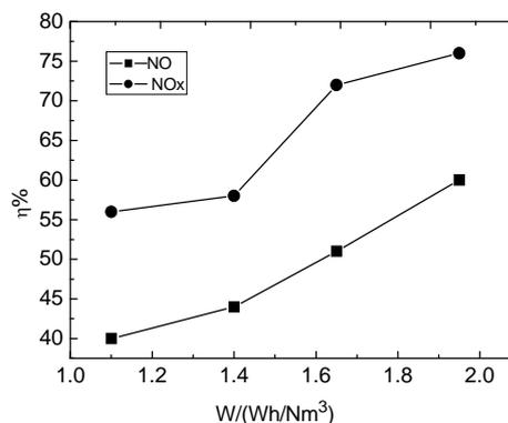
Fig. 10 The removal efficiency of the NO and NO<sub>x</sub> dependent the inserted energy
