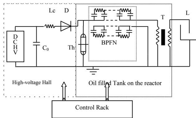
DCHV□high-voltage DC; C<sub>0</sub>□storage capacitors; L<sub>c</sub>□charge inductor; D□high-voltage diode stacks; Th□thyatron; BPFN—Blumlein pulse forming network; T□Pulse transformer; L□Load of the reactor
