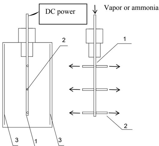
1. Main pipe 2. Pin electrodes with hole 3. Grounded electrodes
