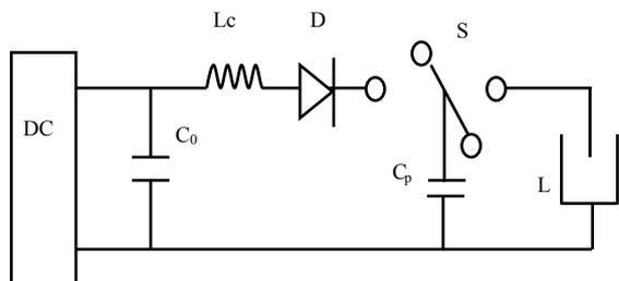
DC- direct power C<sub>0</sub>-energy storage capacitor L<sub>c</sub>-inductance D-diode stack S-rotary spark-gap switch C<sub>p</sub>-pulsed capacitor L-reactor Load
