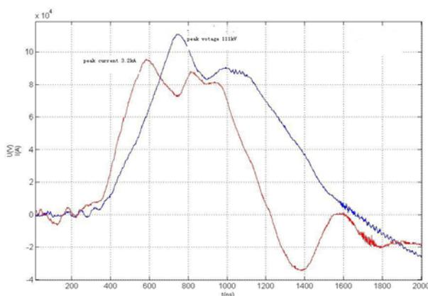
Fig. 7 The voltage (1) and current (2) waveforms of the pulsed power
