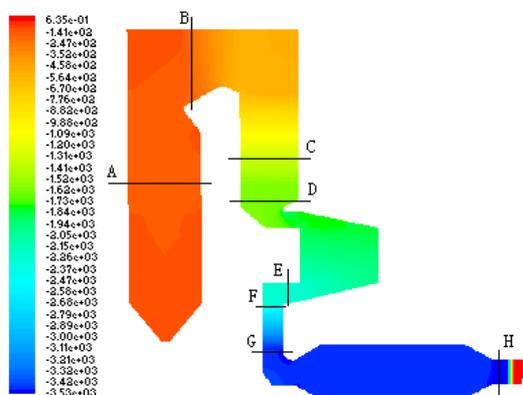
**Fig. 11** Pressure distribution throughout the computational domain
