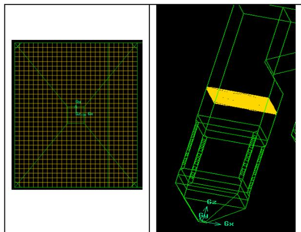
**Fig. 6** Meshing scheme above burner region
