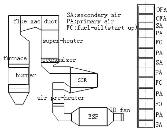
Fig. 1 Schematic arrangement of boiler system and burners
