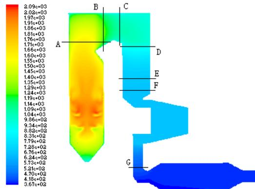
Fig. 9 Temperature distribution throughout the computational domain
