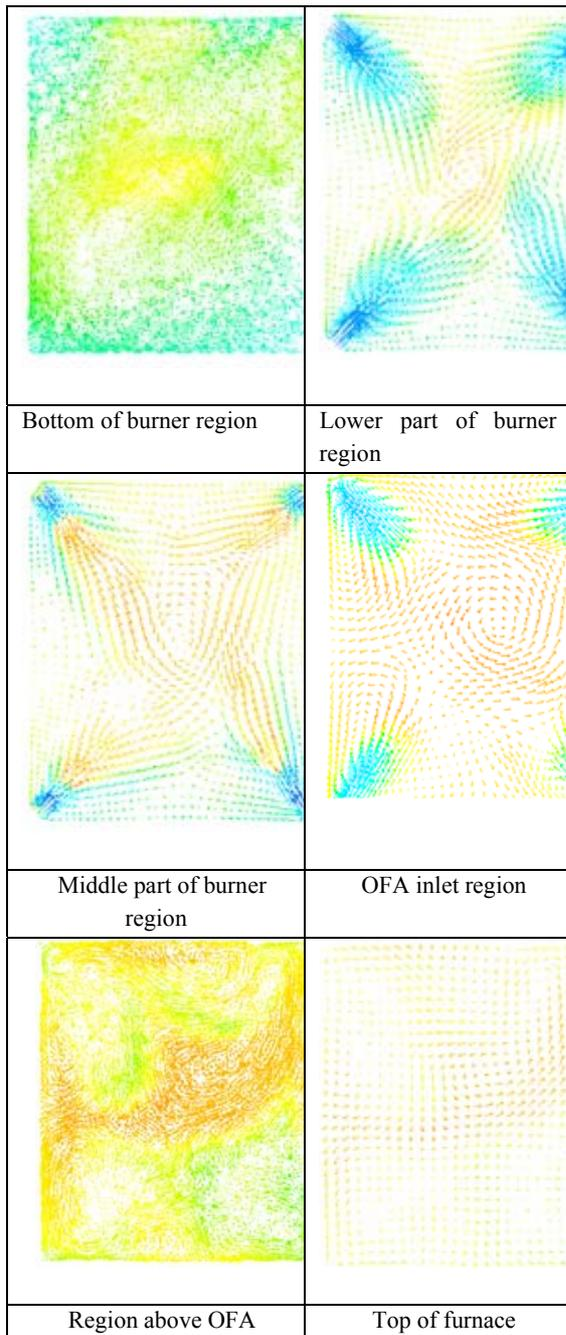
Fig. 8 Velocity vector in the furnace
