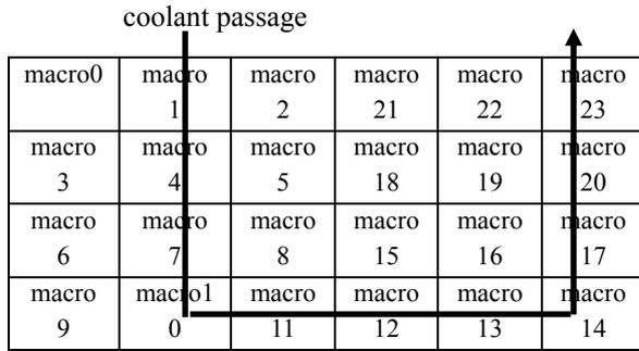
Fig. 7 Core discretized into macros
