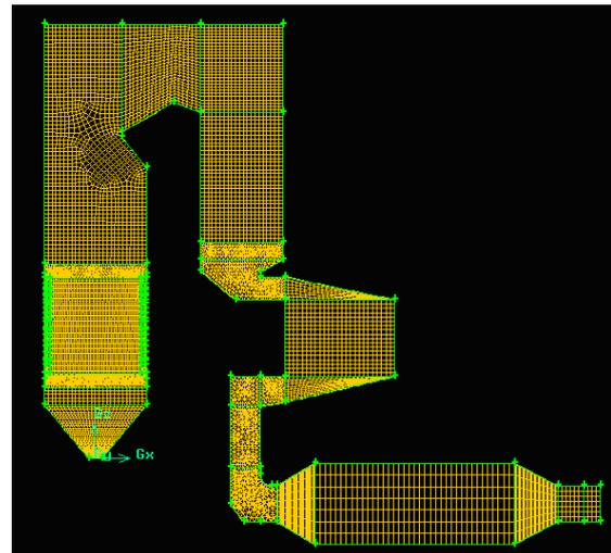
**Fig. 4** Meshing of the whole system
