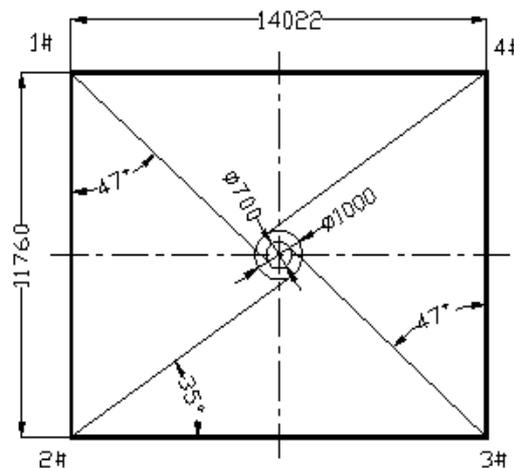
Fig. 2 Orientations of inlet streams
