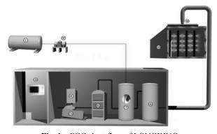
**Fig. 1** FGC chart flow of LONGKING 1 Sulfur storage tank; 2 Sulfur dosing pump; 3 Electrical controlling cabinet; 4 Air filter; 5 Air blower; 6 Air heater; 7 Sulfur burner; 8 SO<sub>3</sub> converter; 9 Inlet duct of ESP; 10 SO<sub>3</sub> injector
