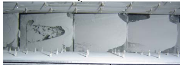
Fig. 6 Photograph of the dust layer deposited on both plates of grounded collection electrode and high voltage in bipolar discharging ESP
