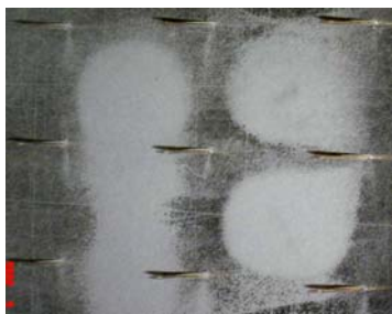
Fig. 11 Photograph of the round silica dust cake deposited on the collection plate electrode
