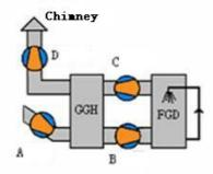
The advantage of location A is that it has little acid corrosion in the condition of high temperature flue, while the disadvantage is the fan abrasion caused by the dust in flue. And the FGD run in the condition of positive pressure, so it requires high in seal, and the location A is the highest point, so the power consumption of the fan is the highest.
