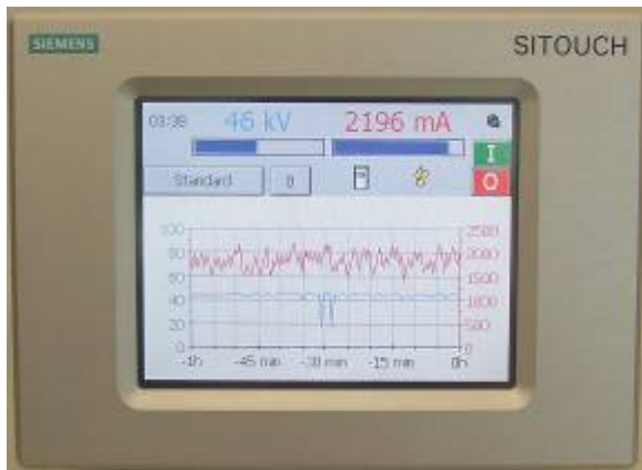
Fig. 5 Operator panel with graphical color display
