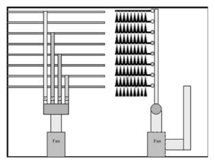
Dust collected in later field has a high content of K<sub>2</sub>O, Na<sub>2</sub>O but little Fe. This kind of dust doesn't have recovery value. So it is discharged from the hopper and not sent to burn again to prevent too many light and fine dust in ESP.
