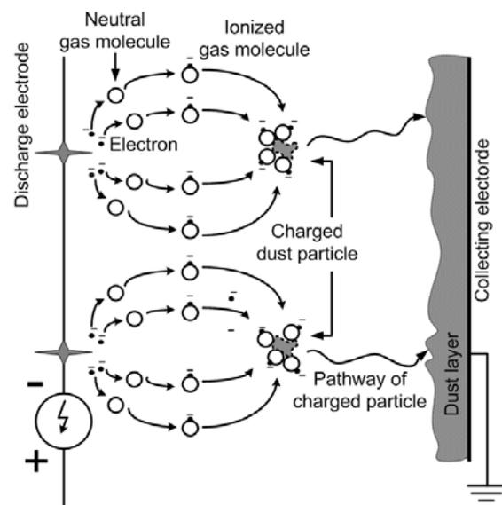
Fig. 2-1: Principle of electrostatic precipitation
