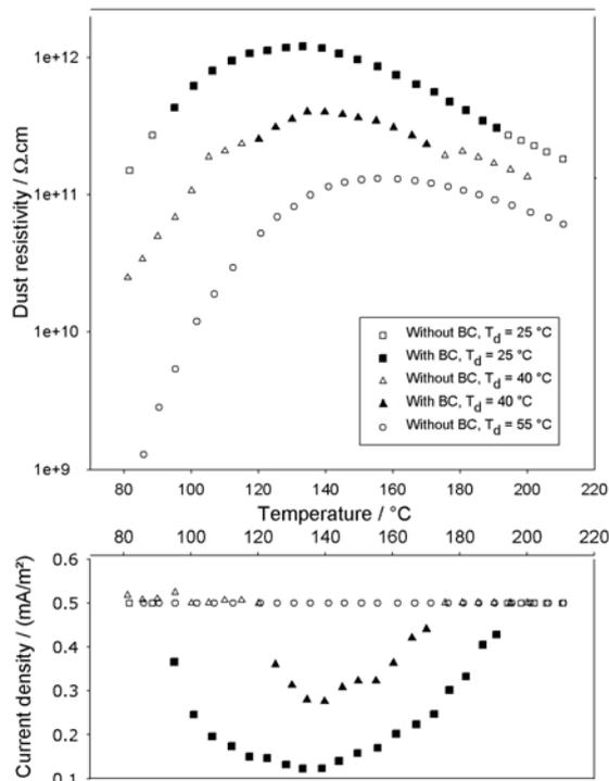
Fig. 5-4: Influence of air humidity on the dust resistivity,  $s = 2.5$  mm, method: plate-plate
