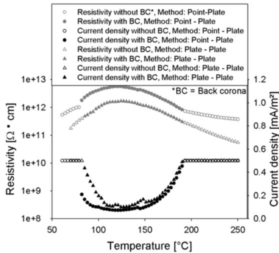
Fig. 5-1: Comparison of dust resistivity measurement methods: point-plate and plate-plate, upper two curves: dust resistivity as a function of measurement method and temperature, lower two curves: current density as a function of measurement method and temperature, layer thickness: 3 mm, air dew point: 20 °C
