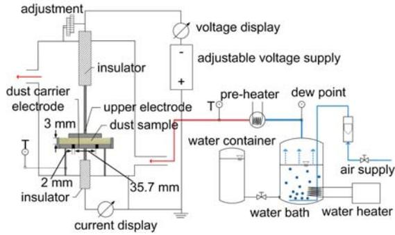
Fig. 4-1: Schematic of the dust resistivity measurement setup
