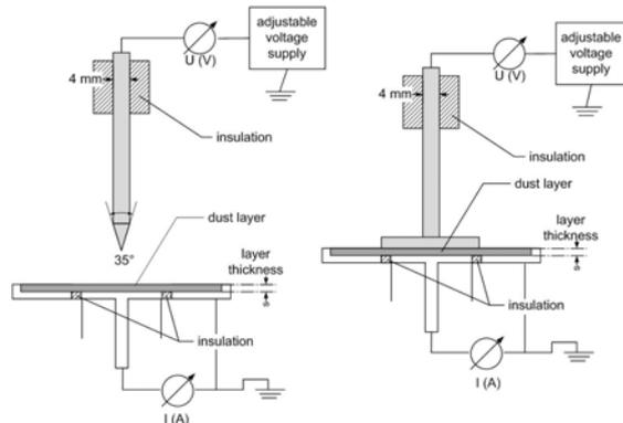
Fig. 4-2: Electrode arrangement in dust resistivity measurement chamber, left: needle-plate setup, right: plate-plate setup
