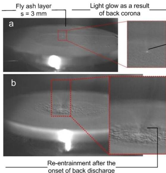
Fig. 5-5: Visualization of back corona in the fly ash layer, inter-electrode distance: 41.5 mm, air dew point: 20°C, a) Visible light glow, b) Blow or re-entrainment of the dust particles
