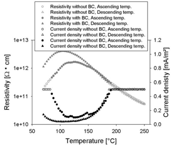
Fig. 5-2: Upper: dust resistivity as a function of temperature, mode of operation (ascending/descending temperature) and humidity, lower: current density as a function of temperature, mode of operation (ascending/descending temperature) and humidity, air point point: 20 °C, layer thickness: 3 mm, method: plate-plate
