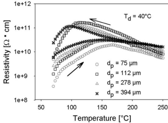
Fig. 5-3: Influence of particle size on dust resistivity,  $s = 3\text{ mm}$ , method: plate-plate
