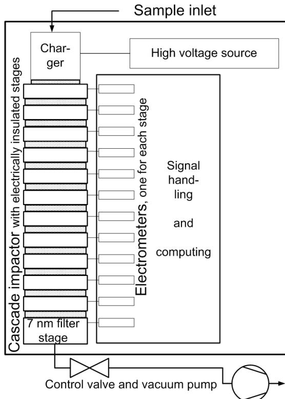
Fig. 3-3: Principle of the Electric Low Pressure Impactor, ELPI
