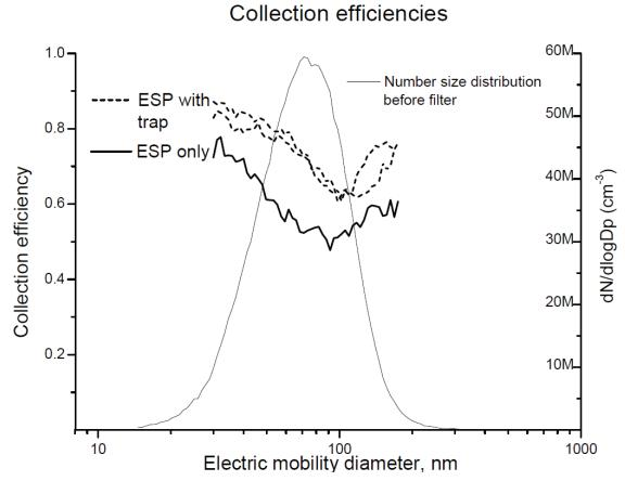
Fig. 4-2: Collection efficiencies based on SMPS data for two ESPs in series with and without the additional particle trap at a gas velocity of 2 m/s through the ESPs
