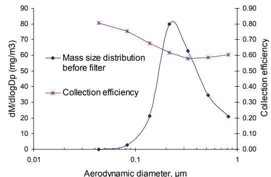
Fig. 4-3: Collection efficiency based on ELPI data for two ESPs in series together with the additional particle trap
