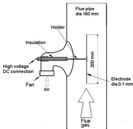
Fig. 3-1: The inexpensive ESP tested for its potential to form part of a precipitator system intended for MW scale biomass plants
