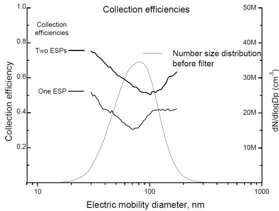
Fig. 4-1: Collection efficiencies based on SMPS data for one ESP respectively two ESPs in series at a gas velocity of 2 m/s through the ESPs
