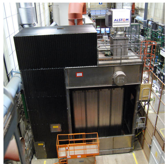
Fig. 3: View of the ESP set-up in the HV-rig with the side cover removed to expose the collecting plates.
