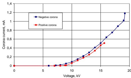
Fig.6 CVC-characteristics of the pilot ESP for different polarity of applied voltage, T ≥ 100°C
