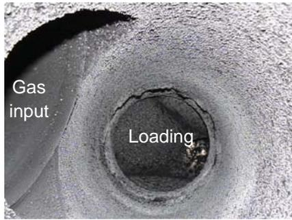
Fig.5 Loading of the ionizer grounded tube
