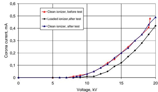
Fig.3 The CVCs of the pilot ESP with clean and loaded ionizer, atmospheric condition
