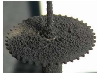
Fig.4 Thick multi-needle disk HV electrode
