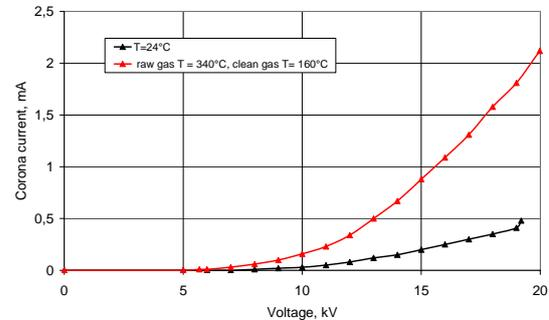
Fig.7 CVCs of the pilot ESP at different gas temperatures
