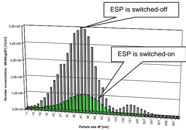
Fig.11 Particle size distribution in the gas flow downstream the electrostatic precipitator, burn-out phase, dilution factor 1:10
