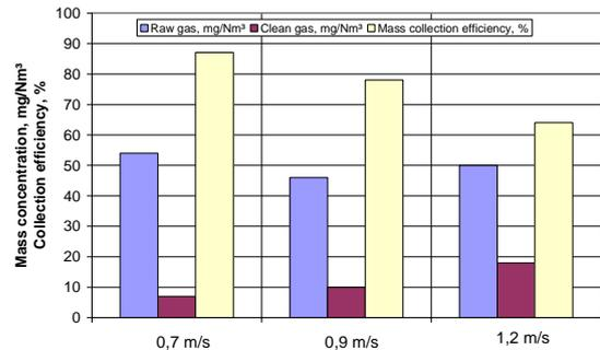
Fig.8 Dependence of the mass collection efficiency on the gas velocity in the ESP
