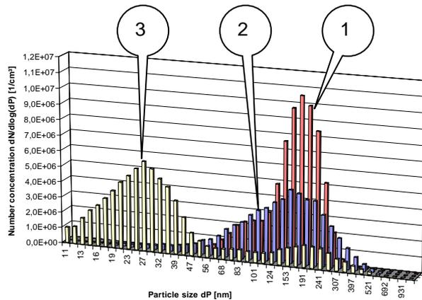
Fig.9 Particle size distribution during different phases of wood-log combustion in a stove: (1) start-up; (2) steady flame; (3) burn-out; dilution factor 1:10
