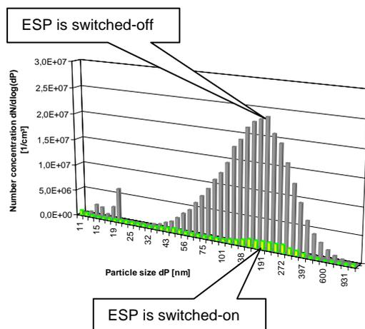
Fig.10 Particle size distribution in the gas flow downstream the electrostatic precipitator, steady-flame phase
