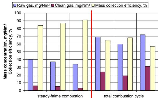
Fig.13 Influence of combustion conditions on the ESP mass collection efficiency
