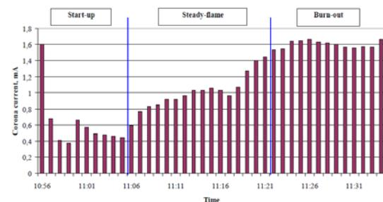
Fig.12 Influence of combustion conditions on the corona current in the ESP
