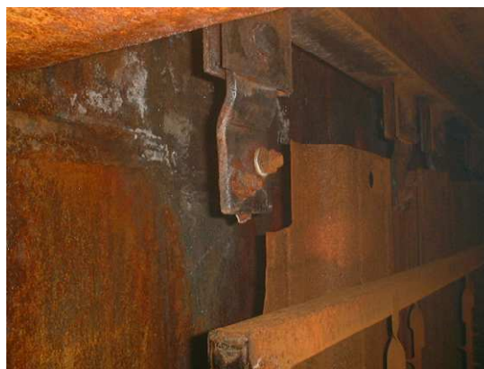
Fig 3-2: Broken Collecting Electrode Due to Hydrodynamic Vibration Caused by High Velocity
