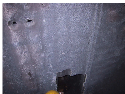
Fig 3-1: Sticky Dust Adhesion on Gas Distribution Plate
