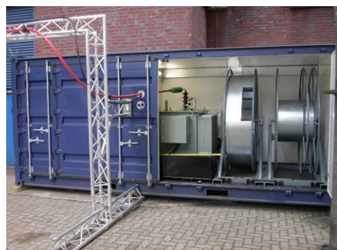
Fig. 5-3: SMPS test installation with single T/R set or SIPREC M container solution
