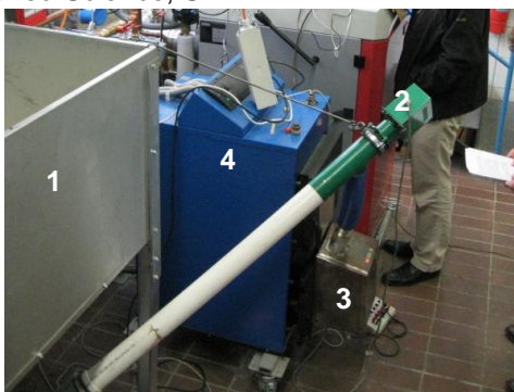
Figure 1: Pellet burner (blue) and wood gas burner (red) in the laboratory of Dezentrale Energiesysteme at the institute for energy technique and motion technique, University of Applied Science, Ulm.
