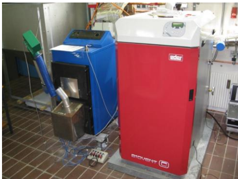
Figure 1: Pellet burner (blue) and wood gas burner (red) in the laboratory of Dezentrale Energiesysteme at the institute for energy technique and motion technique, University of Applied Science, Ulm.
