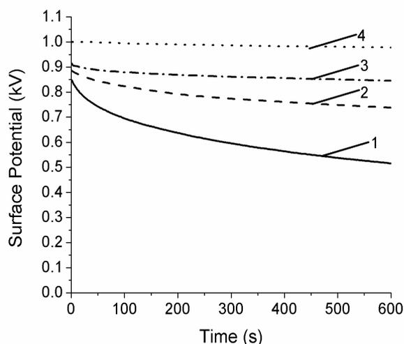
Fig. 8: SPD curves obtained at  $V_g = 1$  kV: 1 – S1 samples and 2, 3, 4 – various S2 samples ( $T_e = 19^\circ\text{C}$ ,  $RH_e = 32\%$ )
