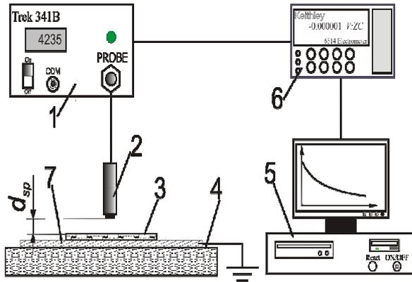
Fig. 4: Experimental set-up for SPD measurement: 1 – TREK 341B electrostatic voltmeter, 2 – TREK 3450 voltmeter probe, 3 – sample, 4 – PVC Support, 5 – computer for data acquisition, 6 – Keithley 6514 electrometer, 7 - grounded plate,  $d_p$  – distance between the sample and the voltmeters' probe
