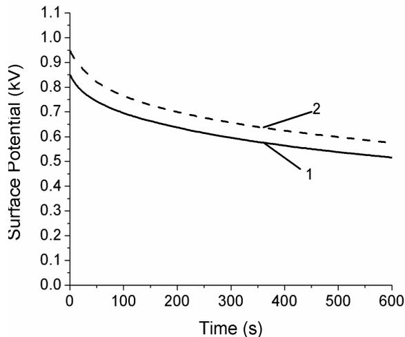
Fig. 7: SPD curves obtained for S1 samples: 1 –  $RH_e = 32\%$ , 2 –  $RH = 15\%$  ( $T_e = 19^\circ\text{C}$ )
