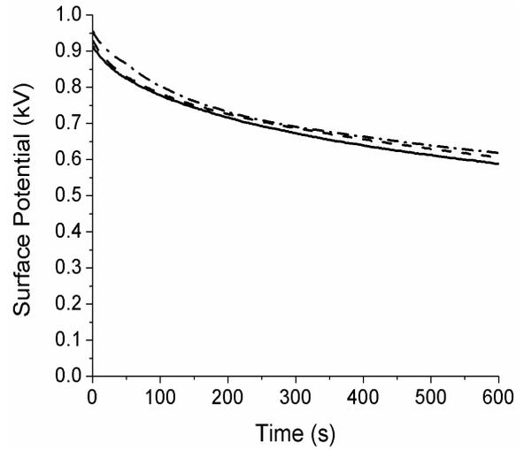
Fig. 5: Repeatability of SPD measurements, for three non-woven PP samples, thermally preconditioned at  $T_c = 70^\circ\text{C}$  and corona-charged at  $V_g = 1$  kV ( $T_e = 19^\circ\text{C}$ ,  $RH_e = 32\%$ )
