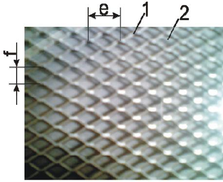
Fig. 3: Grid electrode (1 – wire, 2 – loop,  $e$  – big axis,  $f$  – small axis)
