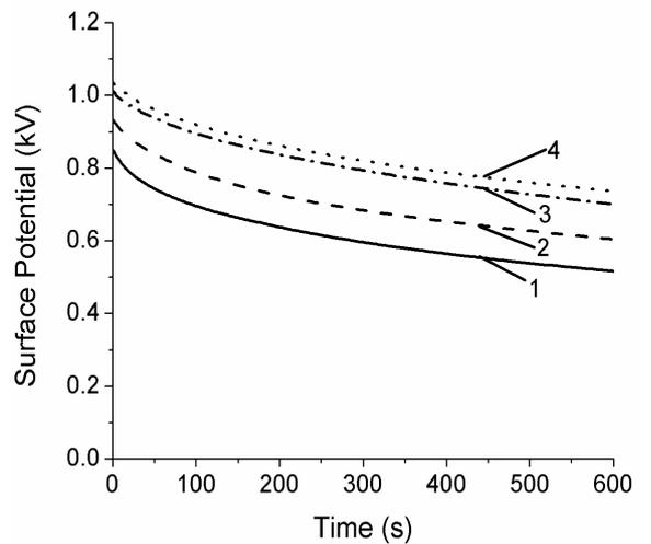
Fig. 6: SPD curves obtained for S1 samples,  $V_g = 1$  kV ( $RH_e = 32\%$ ): 1 –  $T_e = 19^\circ\text{C}$ , 2 –  $T_c = 70^\circ\text{C}$ , 3 –  $T_c = 100^\circ\text{C}$  and 4 –  $T_c = 120^\circ\text{C}$
