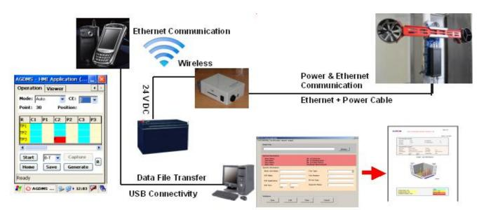
Figure 2 Automatic Gas Distribution Measurement System overview
