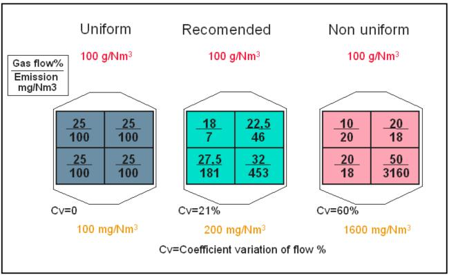
Figure 1 Effects of Gas Distribution in an ESP
