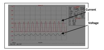
Generally In a control system, the flashover / disruptive discharges are detected through analysis of variations in the waveform of output voltage, output current, input current, etc. These, of course are digital sampling intensity based and hence highly sensitive to be able to detect and take control action for a very low intensity discharge such as spits, etc. Due to the typical waveform, where the effect was negligible, in terms of intensity, the control system was unavailable to detect this.
