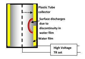
If the plastic tube part is not sufficiently wetted then there is discontinuity in the corona current path, creating surface discharges on the plastic tube collector. This reduces the effective voltage for collection and more dangerously, can seriously damage the plastic tube, because of the localized high temperature. If remain undetected / Unchecked, these could cause holes and deteriorate the collecting surfaces as well as possibly lead to fire hazards, etc.
