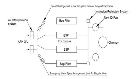
Figure-1 Arrangement of Bag filter retrofit in old ESP casing of a 210 MW boiler
