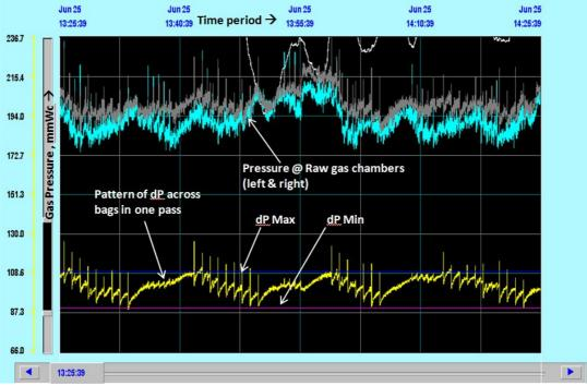
Figure-5 Pattern of dP (in mmWc) - during pulsing cycle
