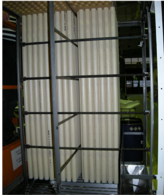
Figure 10. Physical flow model with perforated plastic tubes.
