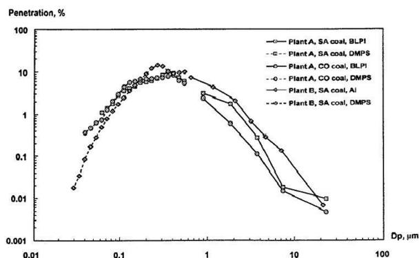
Fig. 1. Particle penetration vs. particle size for ESPs at two different coal-fired plants (from Ref. 16).
