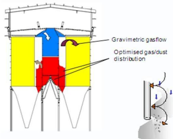
Fig. 3. Principle of gravimetric flow inside the filter compartments to improve settling of the dust.
