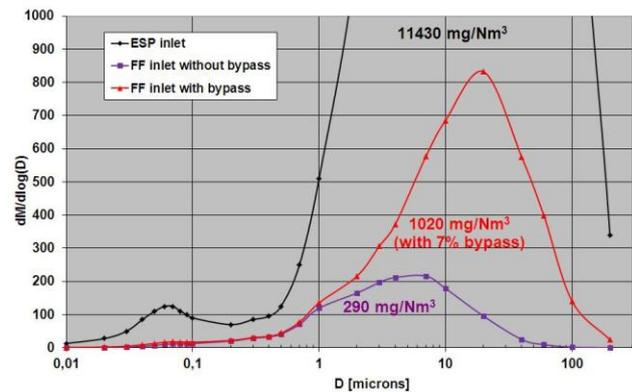
Fig. 5. Estimated particle size distribution at the FF inlet with a raw gas bypass fraction of 7%.
