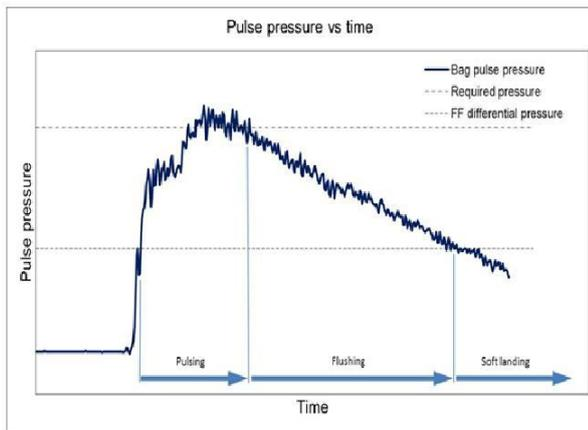
Fig. 2. Pressure profile as function of time for pulse cleaning with the MPC system.
