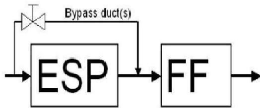
Fig. 4. Sketch of the basic concept with fractional bypass of raw gas to condition the ESP cleaned gas with coarse particles before entering the FF.
