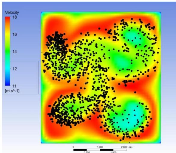
Fig. 6. CFD computation, showing the velocity and particle distribution at a cross section in the main duct between ESP and FF, for one possible layout of the raw gas bypass duct.
