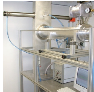
Fig. 6: Test facility, VDI 3926, Typ1
