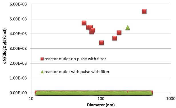
Fig. 7. Particle Size Distribution with filtering (2000rpm, 25% Load, 15kV<sub>pp</sub> and 10 KHz).
