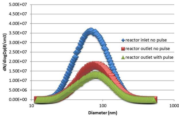
Fig. 5. Particle size distribution (2000rpm, 25% Load, 17kV<sub>pp</sub> and 10 kHz)
