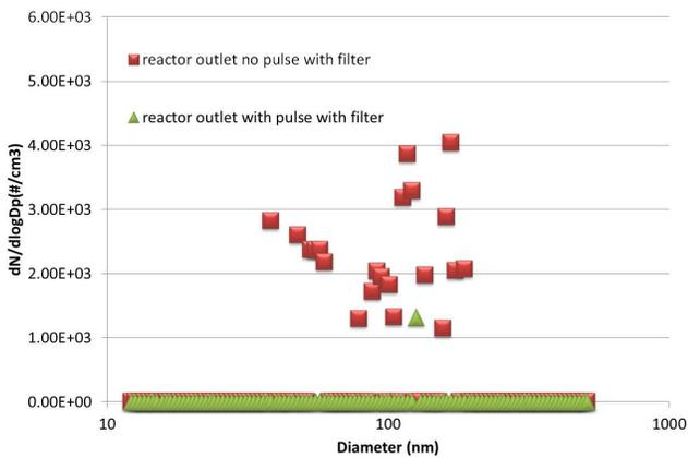
Fig. 8. Particle Size Distribution with filtering (2000rpm, 25% Load, 17kV<sub>pp</sub> and 10 KHz).
