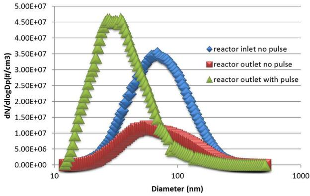
Fig. 4. Particle size distribution (2000rpm, 25% Load, 20kV<sub>pp</sub> and 10 kHz)
