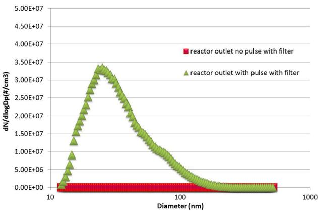
Fig. 9. Particle Size Distribution with filtering (2000rpm, 25% Load, 20kV<sub>pp</sub> and 10 KHz).
