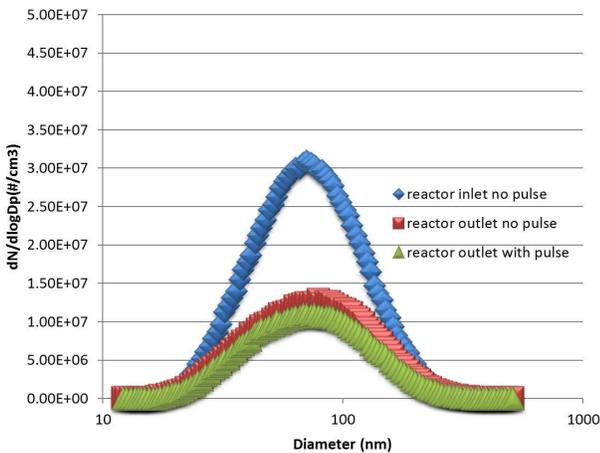
Fig. 6. Particle size distribution (2000rpm, 25% Load, 15kV<sub>pp</sub> and 10 kHz)
